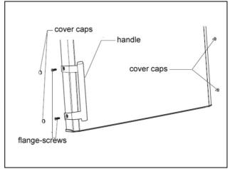
Check if the doors are arranged vertical as well as horizontal, so that a smooth opening and closing of the doors is ensured.
