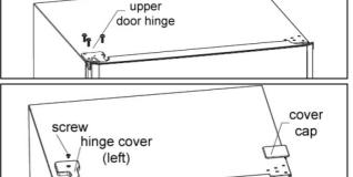
13. Affix the door handles of the refrigerator and freezer door each on the opposite sides. Take off the handles by removing the cover caps of the handles and loosening the below flange-screws. Also remove the cover caps on the door sides and screw the handles into the underlying holes. Put the cover caps of the handles on again. Transfer the cover caps on the exposed holes at the doors each on the other side.
