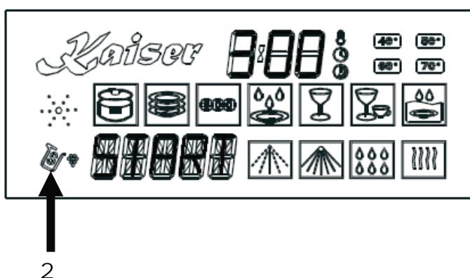
The salt container must be refilled when the salt warning light 2 comes on. Usually, the salt warning light is still on for a certain time after the salt container is refilled with salt and goes out as soon as the salt has dissolved completely.
