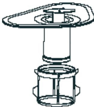
To clean the coarse filter and the fine filter, use a cleaning brush.
