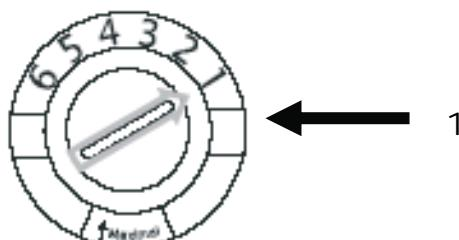
If spots and poor drying are problems, increase the amount of rinse aid dispensed by removing the dispenser lid and rotating the dial to „2”.
