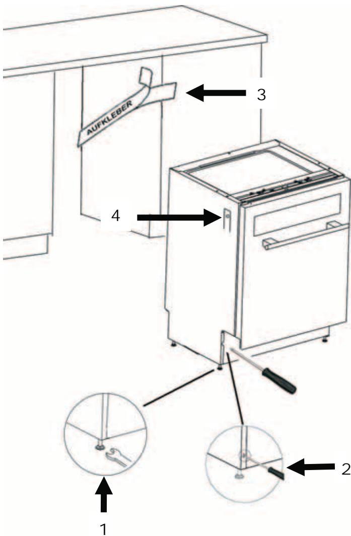
Once the appliance is positioned, level the dishwasher by adjusting the feet 1 and 2 (screw in or out). The inclination angle must not exceed more than 2°.
