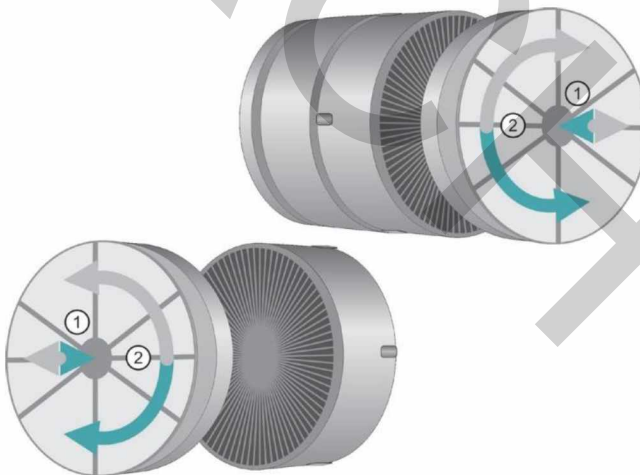
Pic. 14 Carbon filter installation
