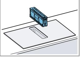
**3.** Remove the four odour filters or acoustics filters, and dispose of them properly.
