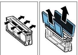
2. Place the individual components of the grease filter loosely in the dishwasher and do not jam them in.
