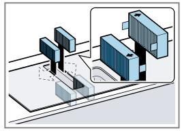
6. Insert the grease filter.
