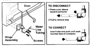
4 Remove the screws from the top hinge. Leave the multi-wire cable inside the hinge. Do not unscrew the ground wire that attaches the cable to the hinge. Lift the door off of the bottom hinge.
