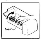
When removing the ice bin, avoid rotating the auger inside the bin. The auger must align with its drive mechanism when the bin is replaced. If you accidentally move the auger, realign by making quarter turns until the ice bin fits back in place.
