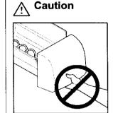
When removing the ice bin, do not grip the ice chute (beneath the front of the bin) as a handle. Surfaces in the ice chute may be sharp.
