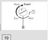
The appliance is switched on by turning the button (B) towards Maxi, and accordingly switched off when the arrow (small triangle) on the button points to the ON/OFF mark  $\,^{\mbox{\scriptsize 0}}$  (the appliance, however, is still under mains power).
