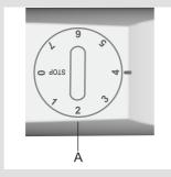
Turn on: rotate the thermostat knob clockwise towards position 7.
