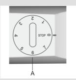
Turn off: rotate the knob back to position STOP (0).
