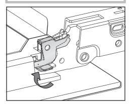
To relock the locking clamps, turn them back up to the horizontal position as far as they will go on both door hinges. Many malfunctions and faults that can occur in daily operation can be easily remedied. Time and money will be saved because a service call will not be needed.
