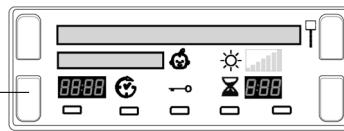
Each press of the Delay button advances the delay setting in 1 hour increments, from: **1h** to **24h**, then **OFF** and then after a couple of seconds cancels the delay.
