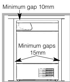
the sides and lateral furnishings or walls. This is to ensure proper air circulation. The appliance must be installed with the rear surface placed against a wall.
