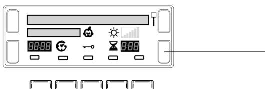
After selecting a programme that has a Timed Dry option, press the Timed Dry button and the display will increment the selected time, each time you press and release the button (*see Start and Programmes*).
