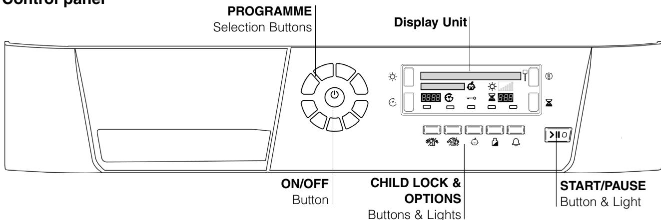
The **ON/OFF** button - if pressed when the dryer is running: If the display shows **TURNING OFF** the dryer stops. If the display shows **PRESS AND HOLD** hold the button and the display counts down 3, 2, 1 and then stops.
