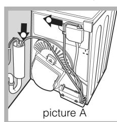
Remove the existing hose from position shown in picture A.
