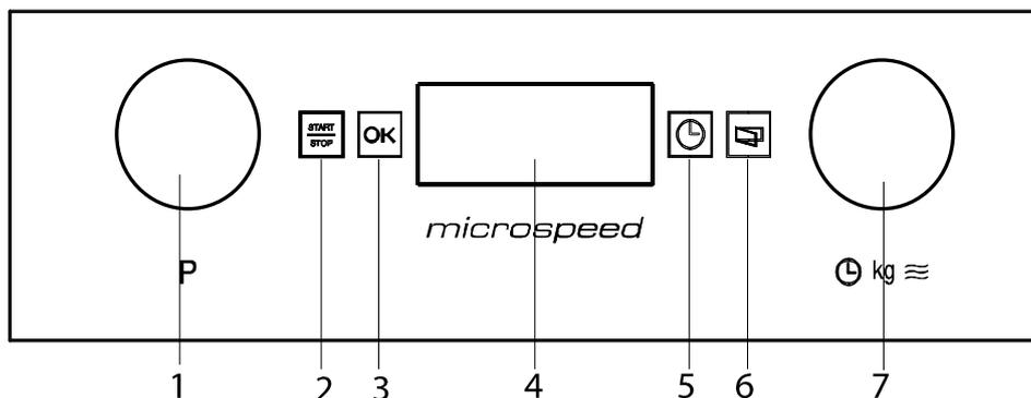
1. Turn the Function Selector knob (1) until the Defrost by Weight function light flashes. The upper display shows the food type "Pr 1" flashing.
