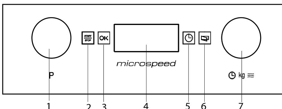
1. Turn the Function Selector knob (1) until the Defrost by Time function light flashes. The upper display shows 10:00 flashing.
