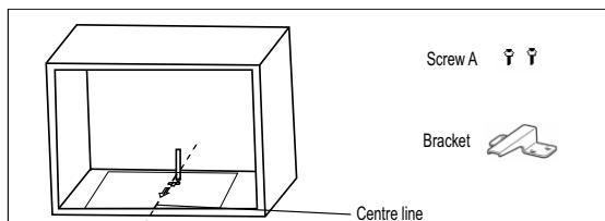
3. Remove the bottom cabinet template and fix bracket with a screw A-3
