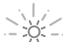
Light button LED
