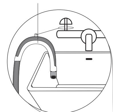
Use the special plastic hose support **4** which is delivered with the appliance.
