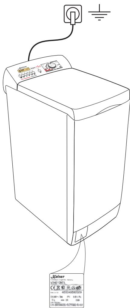
After making sure that the voltage and the frequency values for the current in the home correspond to those on the rating plate and that the electrical system is sized for the maximum voltage on the rating plate, insert the plug into an electrical socket which is earthed properly
